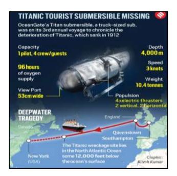
A vessel known as the Titan went missing in the area of the Titanic wreck in the North Atlantic on 19 June 2023. The **Titan** is classified as a **submersible**, not a **submarine**, because it does not function as an autonomous craft, instead relying on a support platform to
